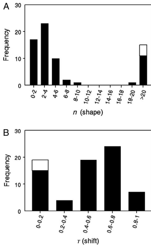
**Fig. 1.** Frequencies of the shape parameter  $n$  (A) and threshold  $\tau$  (B) for the shifted gamma distribution, in a survey of papers examining variability in insect development time. Open bars are the results from Wearing et al. (2004a), which directly fitted the gamma distribution, while the remainder were obtained from studies using the Weibull distribution (see text for details).
